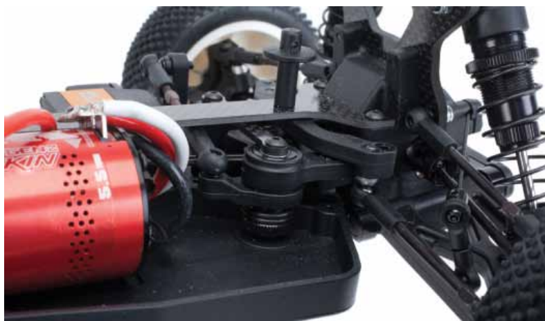
There are two options for the steering Ackermann angle. Anti-roll bars front and rear are standard
