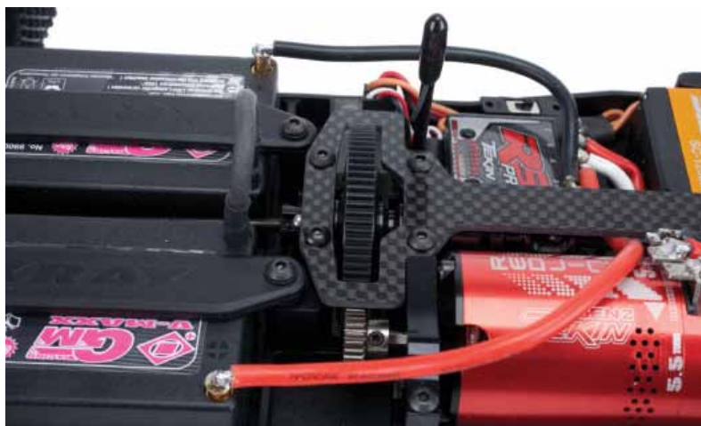
The top deck only braces the front of the XB4 chassis
