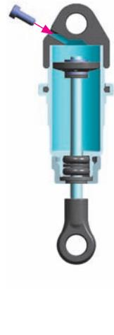
**10** Tighten the screw. The rebound will be at approx. 0%.
