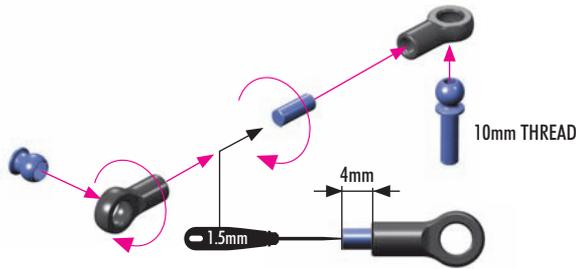
**TIP** Install the pivot balls with Professional Multi Tool (HUDY #183011)
