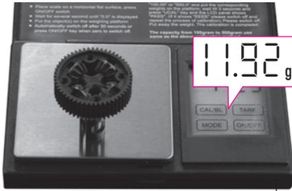
1 Put the diff (without oil) on the scale and check the weight (approximately 11.92g)
