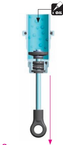
**1** Extend the shock shaft completely. Fill the shock body with the shock oil. For the FRONT shocks (short) use 650cSt oil. For the REAR shocks (long) use 500cSt oil.
