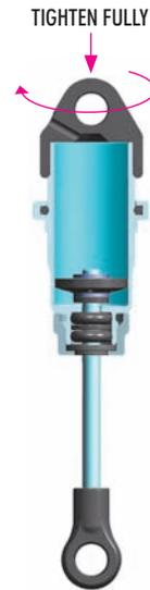
**4** Gently place the shock cap onto the filled shock body and start to tighten the cap. Tighten the cap fully.
