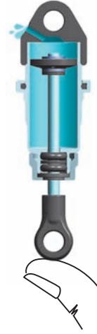
**9** Gently push the shock shaft completely into the shock body. Excess oil will flow through the hole in the shock cap.
