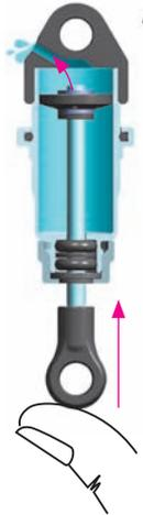
**5** Gently push the shock shaft completely into the shock body. Excess oil will flow through the hole in the shock cap.
