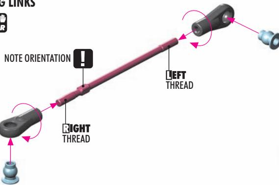
**TIP** Install the pivot balls with Professional Multi Tool (HUDY #183011)
