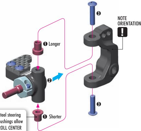
Steel steering bushings allow ROLL CENTER adjustment.
