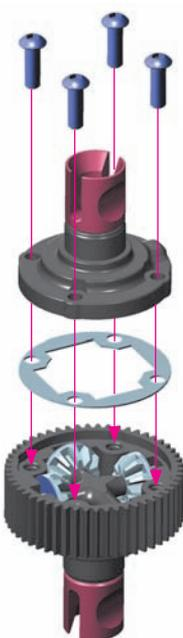
Tighten the screws equally but do NOT tighten them completely.
