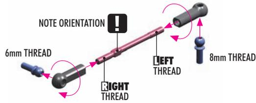
**TIP** Install the pivot balls with Professional Multi Tool (HUDY #183011)
