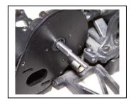
17) From under the car remove the two flat head screws that hold the motor guard. Then, from above, remove the two button head screws that hold the motor guard to the top rear of the transmission. The motor guard and screws will not be needed.
