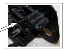
19) Remove the three bolts that go through the transmission and hold the motor plate on. Save the bolts for re-use in A12, but the plate will not be needed.
