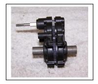
As the case halves come apart, remove and save all of the following parts: Top shaft, spacer, and two 3/8 X 3/16 bearings, Idler gear, two more 3/8 X 3/16 bearings, & idler shaft, Ball differential and two ½ X 5/8 outdrive bearings. You will need all the parts from inside the transmission but the two case halves will not be needed.
