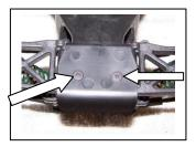
5) Remove the two flat head screws which hold the bulkhead to the chassis. Save them for re-use.
