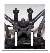
21) From the top, put your wrench down between the wing mounts and remove the two cap head screws that secure the transmission to the shock tower. You should now be able to remove the transmission from the car.
