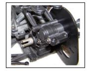
18) Remove the long bolt through the transmission that holds the wing mounts. This bolt will not be needed.
