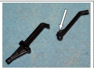
G11) Re-install the top bumper mounts just as they came off using the same bolts. You can throw away the front part which you cut off.
