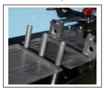
F3) Again, if you are using thread lock, a drop in one end of each 7/8" stand-off. (XF6802) Install one 7/8" stand-off on each side of the battery compartment using two 4-40 X 3/8 flat head bolts. These stand-offs are for the battery strap.
