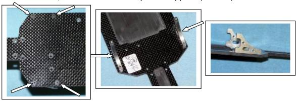
F2) If you use thread lock, put a drop in one end of each stand-off. Install the three 1" stand-offs (XF6801) in the center of the chassis using three 4-40 X 3/8" flat head bolts. These stand-offs are for the top deck.
