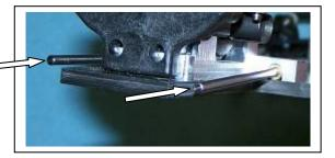
E11) Check the set-up sheet and tuning section to determine whether your control arm inner pivot will be forward, center, or rear. Here we are using arms rear, so the shims go on the front. We use some extra 0.090" transmission shims; shock limiters, flat washers, almost any shim of the correct size will do. If your set-up is arms back, slide the shims on the hinge pins now.
