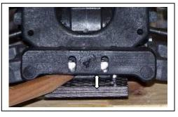
Check the set-up sheet and Tuning Section to determine how much antisquat you will run. There is a packet of small round shims in Bag E, four 0.060" thick (long arrows) and two 0.030" thick (short arrows) (XF3250). This allows 6 different anti-squat settings: 0, .030", .060", .090", .120", and .150" Place two sets of shims between the bar and chassis. Here we show .090".
