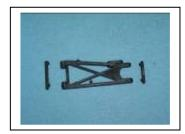
E3) The two arms are identical; when the arms are assembled to the truck, the shocks mount on the rear. However, we reverse the AE hub carriers, putting the right carrier (marked with an "R") on the left arm and the left carrier (marked with an "L") on the right arm. This makes the camber links line up better.
