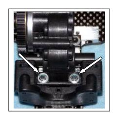
D11) Place a flat washer over a 4-40 X 3/8" screw, put the screw on your wrench, and fit it down between the transmission and the motor plate to secure the left front tab. Be sure the shim is in place (left photo). Now tighten both bolts and both nuts.
