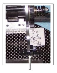
D9) We'll do the easy one first. Place a flat washer on a 4-40 X 3/8" cap head bolt, insert the bolt through the hole in the right front transmission tab, through the shim, and screw it finger tight into the cradle.
