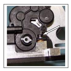
D10) In the rear, place flat washers over the two studs which should protrude through the rear transmission tabs.
