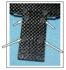
D3) Now install the transmission cradle (XF5030). If you use thread lock, do only the two front holes. The two rear holes are not tapped, but you will want to twist the 1" bolts to help the cradle slide down. You want to twist a little bit on each bolt in order to keep the cradle level as you install it. "Walk" it down. Don't let it get on a large angle as in the left and center photos. Keep it level, as in the right photo.
