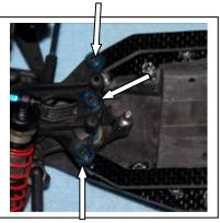
C5) Put the front bumper on the truck using the two 4-40 X 5/8" flat head bolts you saved.
