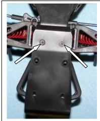
Position the nerf bar over the front brace and on the bumper surface just as it was on the SC10 and secure it with the four 4-40 X 3/8" cap head bolts you saved.
