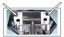
C2) Now use the two 4-40 X 3/8" cap head screws (XF6001) to attach the rear of the front decks (XF1500) to the lower part of the top deck supports (long arrows). Leave these screws finger tight for now so the front of the parts will move a bit. The hole in the front should line up with the stand-off (short arrows) but no screws in here yet.
