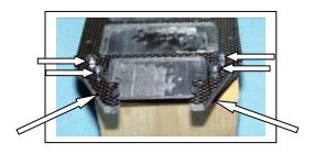
B4) Take the nose piece (XF1002) out of Bag B and check it for flashing, especially at the rear and on top of the post. We need good snug fit with the chassis and especially where the top deck fits on the post.
