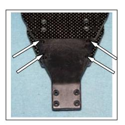
B6) From above the chassis, place locking nuts on the two rear screws that hold the nose piece (short arrows). If you use thread lock, place a drop in one end of each 13/32" stand-off (XF6803) and screw that end onto the front two screws (long arrows). Tighten the stand-offs securely.
