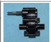
A21) Install the 4-40 X 3/8" cap head bolt (XF6001) in the lower corner of the trans case, just finger tight for now to hold things together.
