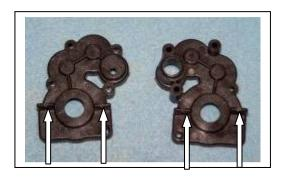
A14) Install a 3/16" X 3/8" rubber sealed bearing (XF6200) all the way into the top shaft boss in the left transmission case half (short arrow) and a 3/8" X 5/8" rubber sealed bearing in the boss for the differential. The Team pushes them in with the shank of an Allen driver or, better yet, with a socket. See Inst. A16.
