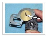
A25) Put a slipper pad on the 78 tooth spur gear supplied in your Kit – the larger one from the SC10 will not fit. (left & center photos). The hex of the pad fits into the molded hex in the gear. Now turn the transmission so the top shaft with slipper plate is facing down. Hold the plate on with your thumb and slide the spur gear, pad side up, onto the shaft so the pad & gear are tight against the plate. Keep pressure on the spur so the pad
