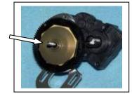
A27) Install the spring on the shaft so it goes around the slipper plate's hub, then place the black retainer over the spring, flat side up. Install the 5-40 nut to hold it all together, tightening until there is one thread of the shaft showing. Final adjustment later.
