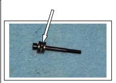
A9) Put the thrust bolt, with thrust bearing, on your Allen driver, and install the bolt into the female outdrive (center photo). Leave the driver engaged in the bolt through step A 10. Now put the diff gear, with balls and bearing, over the bolt so the diff balls contact the diff ring (right photo).
