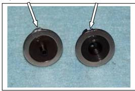
A5) Re-install the diff balls and one diff bearing into the diff gear. Put a small amount of diff lube on one side of each of the balls. We used too much in the photo so you can see the lube. You need surprisingly little lube, and excess is just thrown off inside the transmission case. Many X Factory Team drivers use B-Fast Pro Lube.
