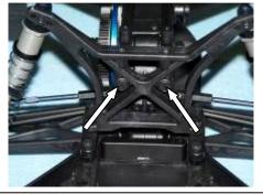
11) Remove the long bolt and captured nut that hold the two pieces of the bumper together.
