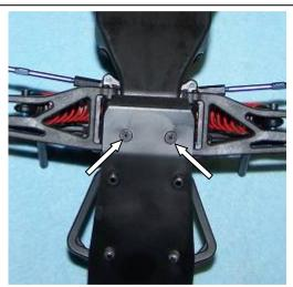
7) Still working beneath the chassis, remove the two flat head screws which hold the bulkhead to the chassis. Save these screws for reuse.
