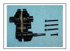
21) Remove the transmission components. The case will not be needed, but you will need the top shaft and spacer, two 3/16" X 3/8" bearings, idler gear with its two 3/16" X 3/8" bearings and shaft, and the differential assembly. The outdrive bearings will not be retained.
