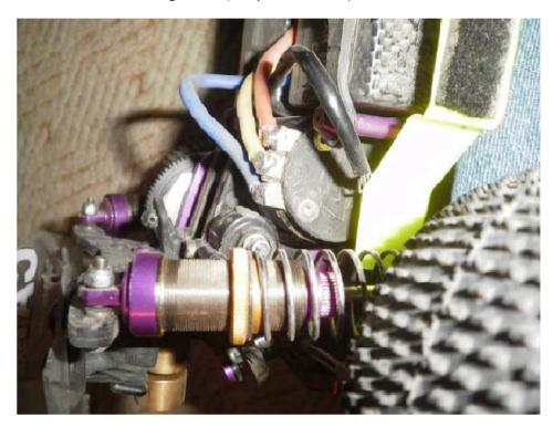
Cat rear driveshafts, (longer than kit) spaced in 2mm with a cat front wheel washer used instead of the kit purple one for wheel mounting. Drive cup cut down accordingly to allow full suspension travel. (see pics). This brings the inner dogbone closer inline with the hingepin and allows the rear suspension to be more supple and allow the rear to roll more
