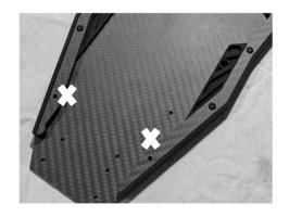
The two front holes do not need screws yet.
