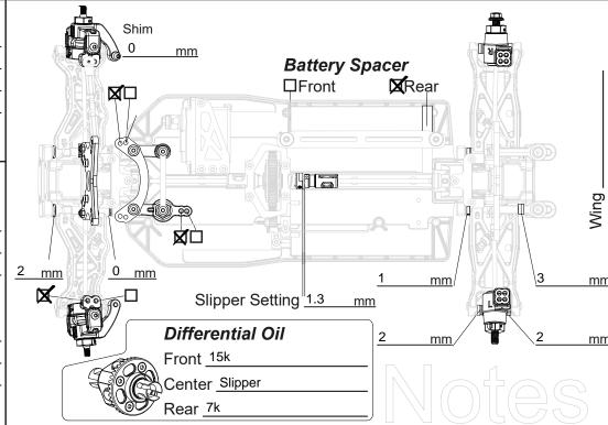
When using the AE 3 pad slipper, you will need to open the center hole. You will need a total of 4 AE slipper pads. 3 on one side and 1 on the other. The side with 3 pads needs to face the rear of the car.
