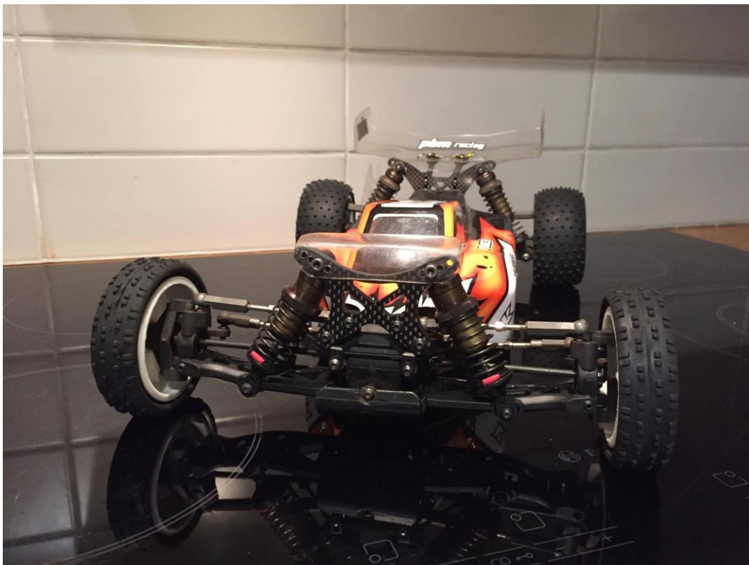
Shaun Thompson's ZX6.6 with Yokomo front gullarms and Kyosho caster blocks and steering arms.
