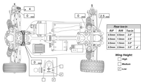
Notes We changed the setup throughout the races because of the changing track conditions, the grip kept increasing, this is the setup we ended up with.
