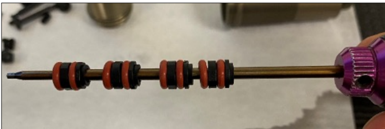
1. Orient bushing and O-rings onto shaft
