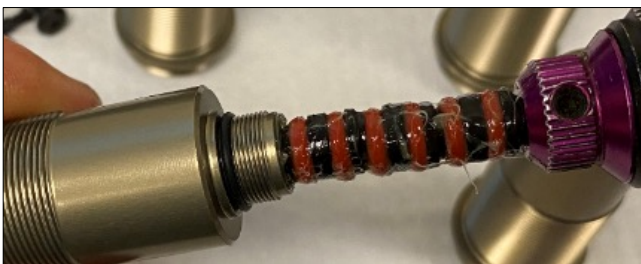
3. Insert assembly into shock body
