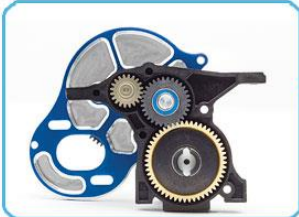
3-gear transmission with lightweight V2 aluminum top shaft
