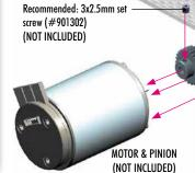
Some motors do not have a chamfer on the motor housing. If your motor does not have a chamfer on the housing and you want to use a small pinion, the motor may touch the top deck. Use a moto-tool with grinding bit or file to remove material from the top-deck; this will allow the motor to be moved closer to the spur gear.
