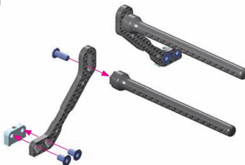
The optional horizontal rear body mounting has proven beneficial for medium- to high-grip conditions, and especially on technical tracks. The horizontal mounting improves the direction change of the car, improves steering response, and improves rotation. However, rear grip is reduced. This is particularly useful for spec classes such as Stock and Super Stock. The kit carbon mounts allow for the height of the horizontal posts to be adjusted.
