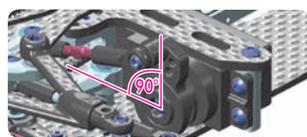
Attach servo arm to servo output shaft using screw from servo. Servo saver must be perpendicular to chassis when servo is in neutral.
