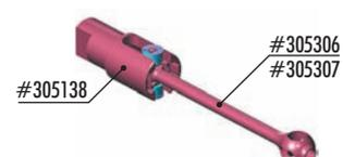
The optional ECS ball-bearing driveshafts feature a new ball-bearing assembly at the inner end of the driveshaft where it inserts into the outdrive. The friction between the driveshaft and the outdrive is greatly reduced, which gives smoother handling especially on fast direction changes such as chicanes. The reduced friction also helps to increase cornering speeds.
