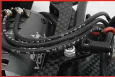
We fitted thin 16AWG wires from the speed control to the motor for greater flexibility
