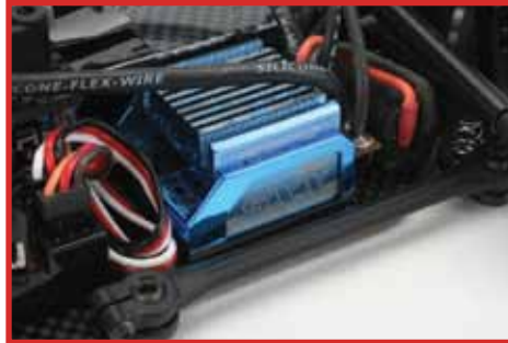
LRP's SXX StockSpec Version 2 was our choice of speed control, connected to a Team Orion 10.5T
