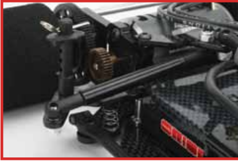
Damper tubes slow down the side-to-side movement of the chassis
