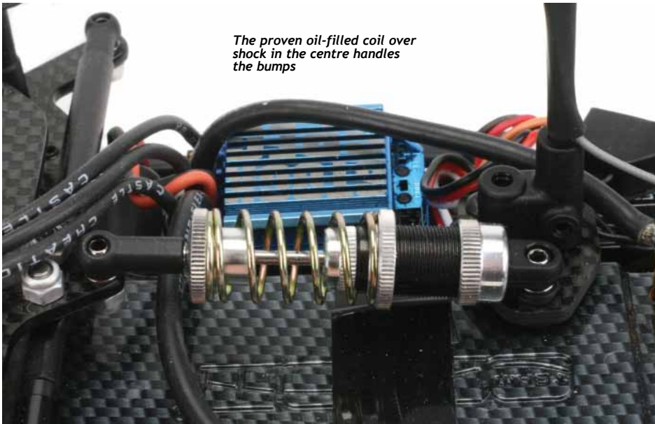
We fitted thin 16AWG wires from the speed control to the motor for greater flexibility
