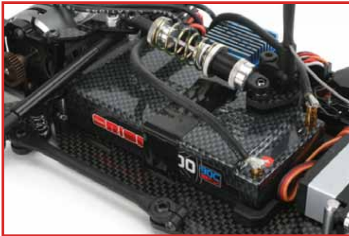
The Team Orion 1S LiPo locates down the right-hand side of the chassis
