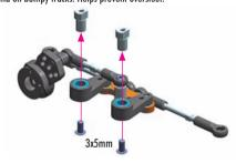
NOTE: The floating steering arms are mounted on the graphite servo holder in the Final Assembly page 33/step 1.
