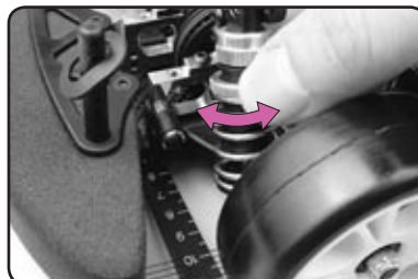
Changing front spring preload
