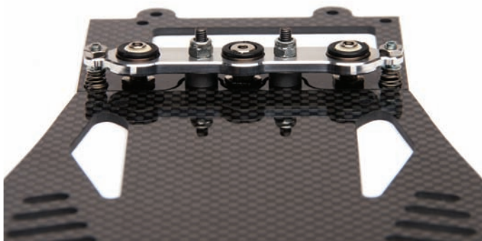
Above: Rear pod linkage, which controls side-to-side and forward suspension movement area
