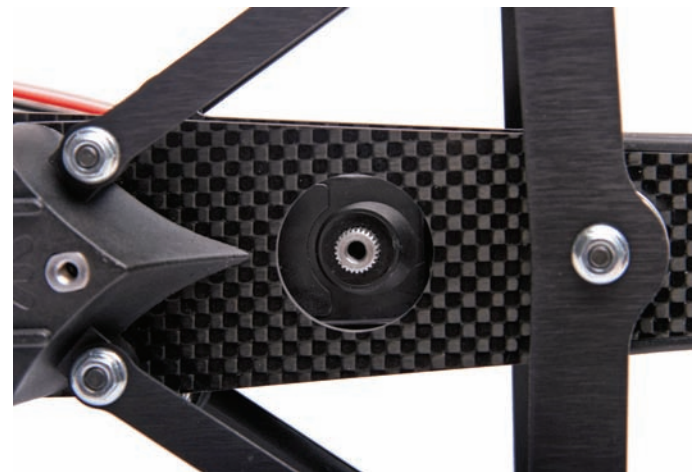
Below: The wide low front wing... it doubles as a bumper!
