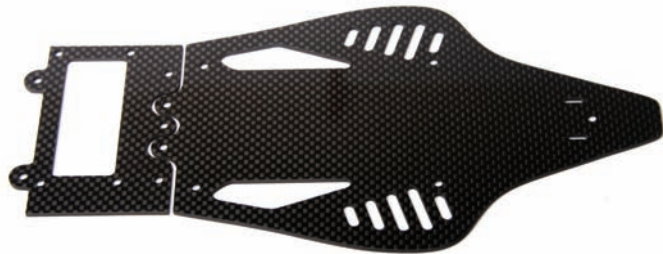
Above: 2 mm thick carbon high-gloss chassis and the motor/pod plate
