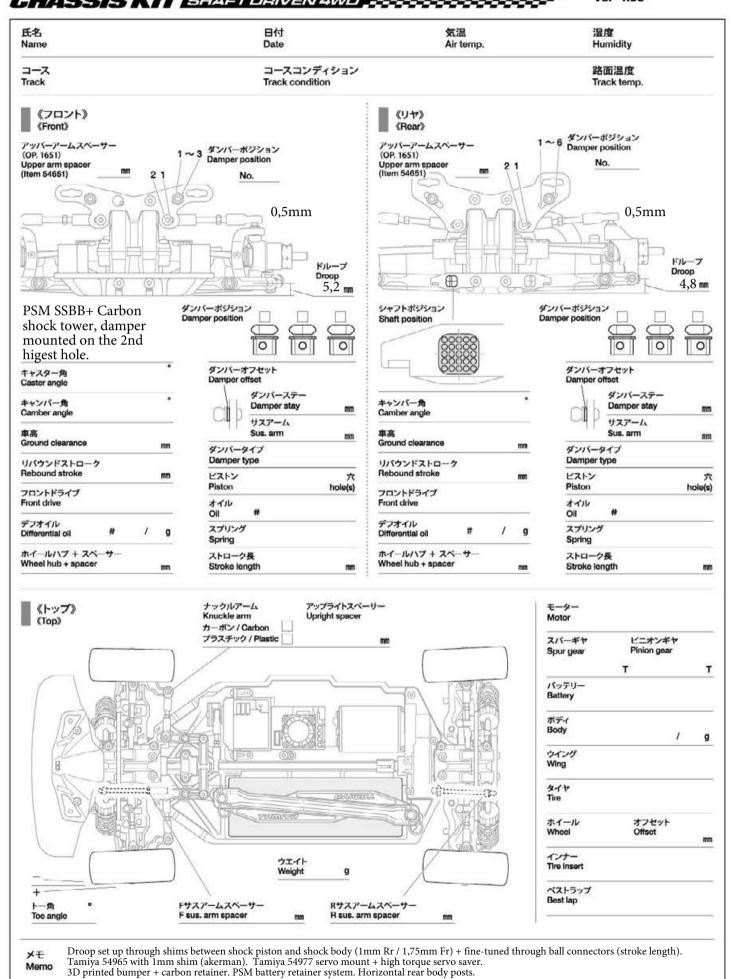
HW Xerun V3.1 ESC with 20° boost timing (no turbo). 40mm fan on the motor. Ratio around 4. Car is slightly loose at the rear to allow placement in turn. Very strong front end and good traction.
