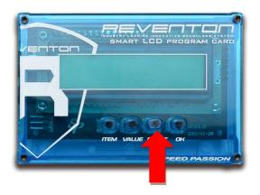
4. The LED program card will be display "- - - - ". The LCD program card will display "FIRMWARE UPDATE ". Release the "RESET" button and launch the "Speed Passion Reventon PC Interface" program.
