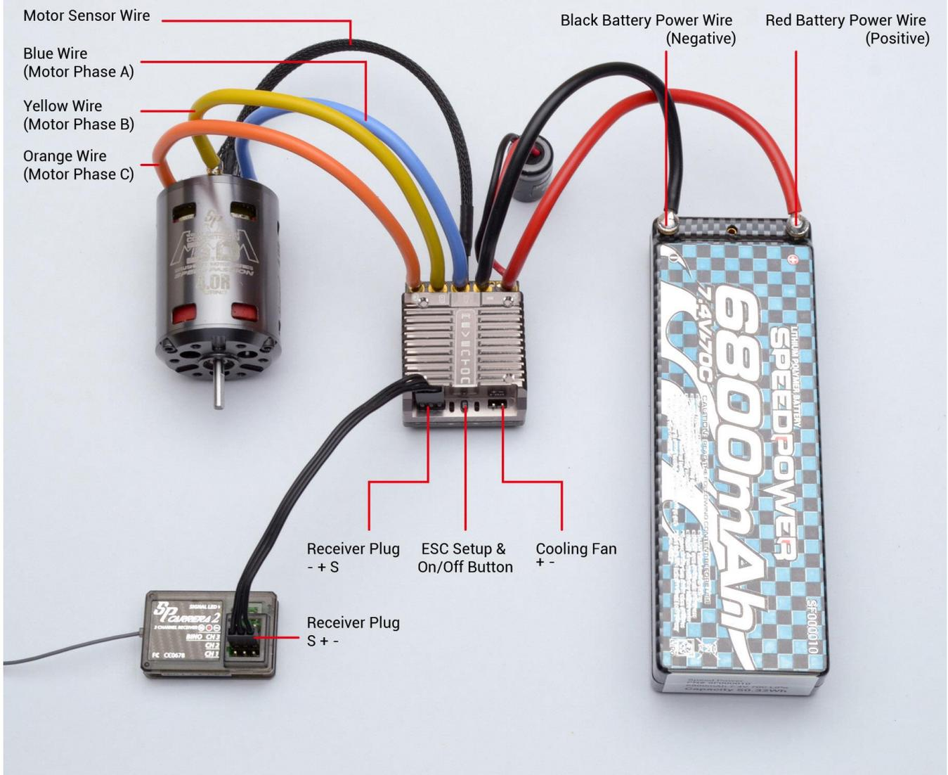
**Picture A: Wiring with a brushless motor**
