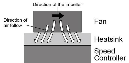
9.1 **Heat sink fan (6V):** The 6V fan is necessary when using battery packs is more than 6 cell NiMh/NiCd or 2s Lipo. It is mounted to the heat sink of the ESC. It helps to cool the ESC with downward airflow. The picture on the top side shows the installation.
