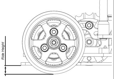
Using these Eccentrics for the foam diameter stated will give the kit rear ride height setting of approximately 3.5mm.
