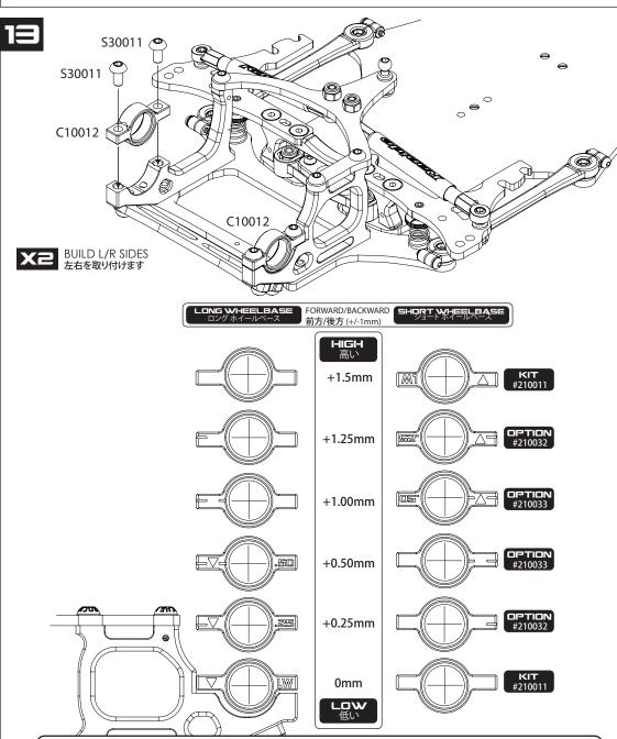
RAPIDE P12/P10 IS ADJUSTABLE MAIN SHAFT POSITION TO FORWARD/BACKWARD (+/-1mm), AND THE HEIGHT OF MAIN SHAFT +/-1.5mm BY DIFFERENCE ORIENTATION OF ADJUSTER.
