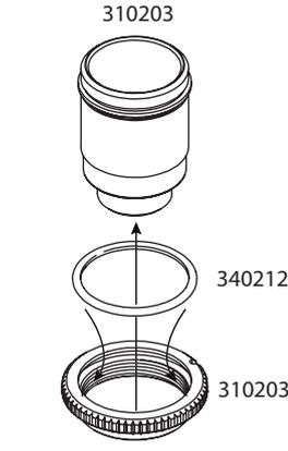
**!** O-RING INSERT INTO THE GROOVE
