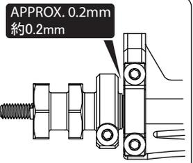
THE AXLE MUST HAVE A SMALL AMOUNT OF SIDE PLAY. ENSURE THE SHAFT IS ROTATING FREELY.
