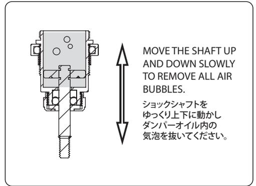
MOVE THE SHAFT UP AND DOWN SLOWLY TO REMOVE ALL AIR BUBBLES.
