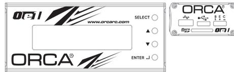
To begin, connect the battery wires to a charged battery, then connect supplied 4pin wire (200mm) to the ESC setting port (4pin port) and Program Card. Turn on the ESC and the Program Card will activate automatically. Note that the screen will show "Loading..." during initialization - indicating that the ESC is copying the current setup in the ESC to the Program Card. Once loading is completed, the screen will show "ORCA Oe1" and "Program". You can now begin programming your ESC.
