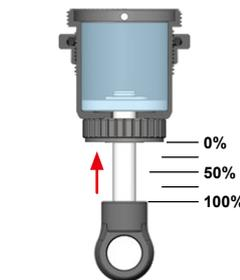
To adjust the rebound amount of the shock, push the shock shaft in to the required.
