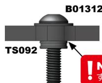
Remove screw (B01312) after press-fitting M3 Press Nut (TS092).
