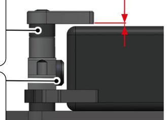
**! The front-back mounting position of the battery is adjusted by the thickness of this shim.**
