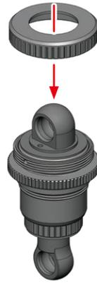
Gently place the shock top onto the shock membrane and allow the excess oil to drain under its own weight.
