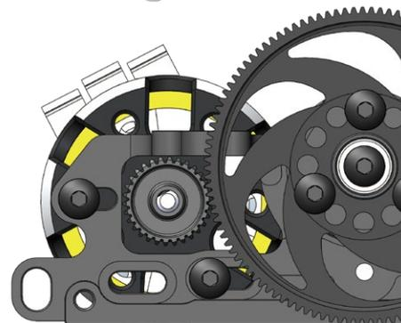
**By changing the position of the motor mounting holes, the motor can be mounted approximately 0.5 mm higher.**
