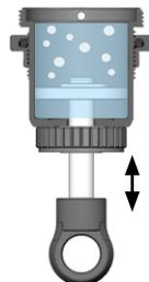
Move the shock shaft up and down to let the air bubbles escape from the oil.
