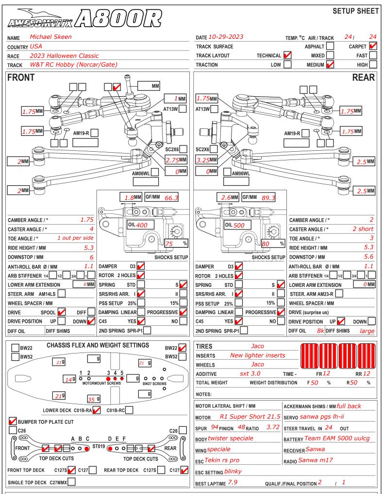
**COMMENTS:** Carbon front bumper top plate with brace cut out. 1.75 shim under rear body mount brace so it sits flush, and a c26 under this to stiffen the rear bulkhead flex (this sits on top of my split upright cf mounts for vertical body posts. 1.5mm front and rear c45.
