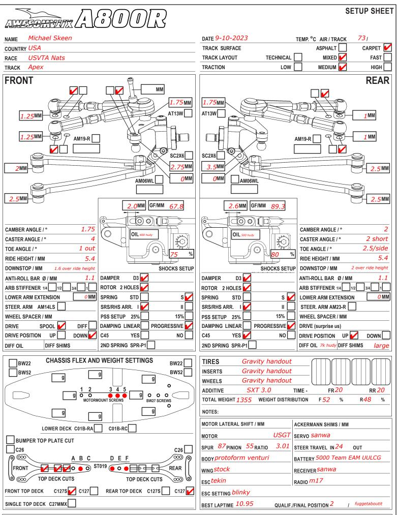
**COMMENTS:** Custom front carbon fiber bumper plate that braces against bulkhead but doesn't connect to bulkheads. Custom M braces 2mm thick designed to flex more than c26 on front bulkheads. 40g tungsten putty added under front bumper. Custom 1.5mm rear damper c45 brace.
