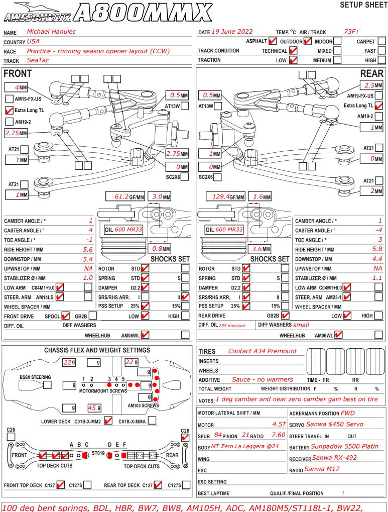
100 deg bent springs, BDL, HBR, BW7, BW8, AM105H, ADC, AM180M5/ST118L-1, BW22, BSWorks Fan Mount, WTF3010BH9, Mxlr 23t horn; Diff measured with Arrowmax v2 meter Remaining tests - retesting chassis flex with top decks / rear C26 / AM105H; ESC software; 15deg front pss; front diff with ear plugs; rear 110 springs
