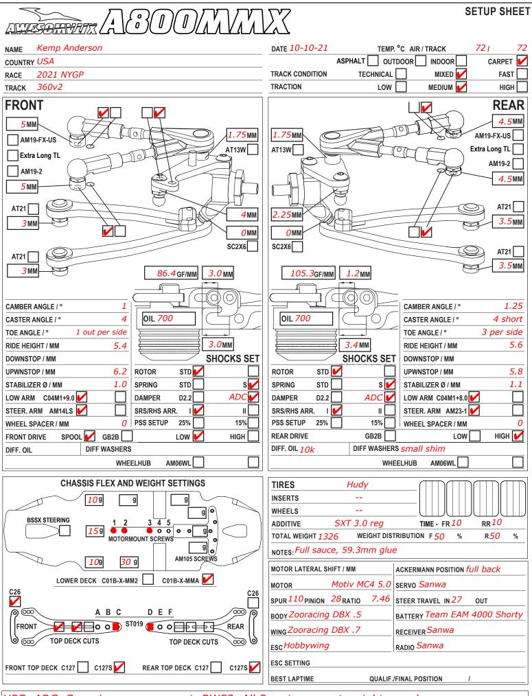
*HRB, ADC, One piece servo mount, BW52, All 3 motor mount weights used Arrowmax oils used in diff and dampeners New AMX chassis used (no holes for short arms, battery shifted forward) To make car feel more in the track go to B and E holes in top decks*
