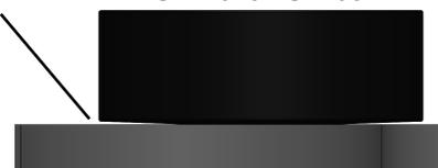
The engraved sides of **ST110** and **ST105** are flat. The opposite sides are chamfered.
