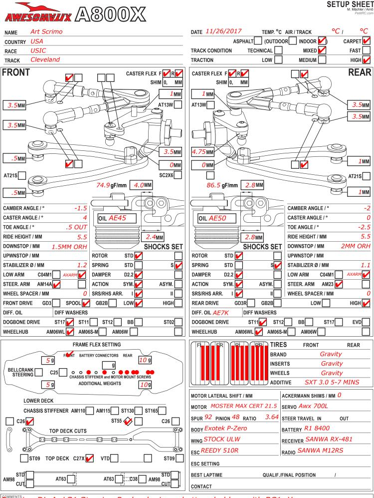
Running DL-A, LS1 Steering Rack, aluninum battery holders with BC1, Xray servo saver, Lundsford screws and turnbuckles, Avid Ti ball studs and Xray ball cups. Car was very good all weekend even when grip got really greasy.
