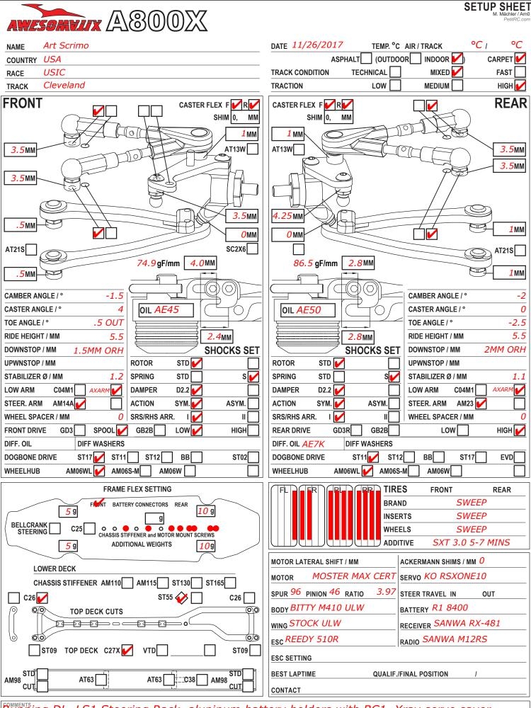
Running DL, LS1 Steering Rack, aluninum battery holders with BC1, Xray servo saver, Lundsford screws and turnbuckles, Avid Ti ball studs and Xray ball cups. Car was very good all weekend even when grip got really greasy.
