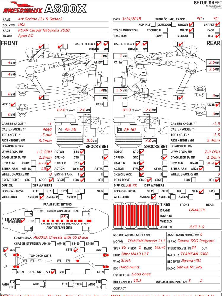
Belicrank Steering, No DL, Xray Servo Saver, MRT Transponder next to receiver, SXT 3.0 for five minutes full sauce, 59.5 Front glue, 58.5 Rear glue, IFJ in Front, Progressive front springs at 4.0mm.
