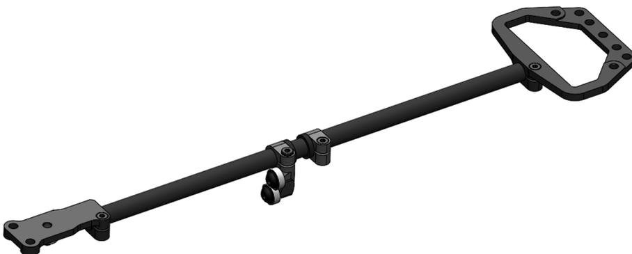
The top surfaces of AM46 and AM40 plates should be parallel. Align them on the flat board before SC2X6 screws tightening.
