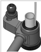
Oil filled steering blocks also need to a space for exessive oil to be removed, to bleed the steering block. Like the rear damper, use a needle to create a gap between the o-ring and the steering block to allow excess oil to be removed.
