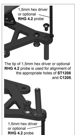
Alignment of the appropriate holes of ST1208 and C1205 for camber settings.
