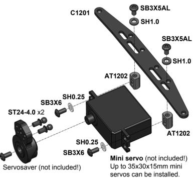
Note: ST24-4.0 are 4.0mm ball studs. ST24-4.0 fit P1213 4.0mm ball cups.
