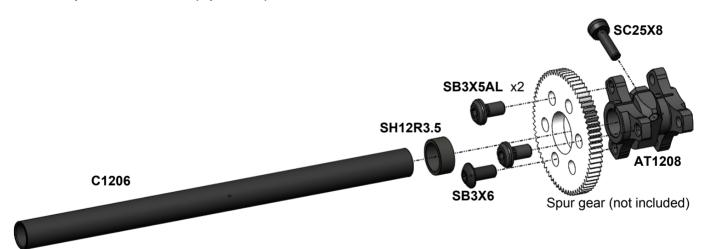
**Note**: Optional **ST1212** steel axle can be used instead of **C1206** carbon axle.
