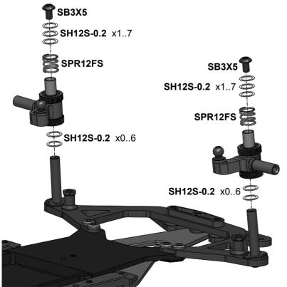
**SH12S-0.2** 0.2mm thickness shims are used to set the front spring preload and the front ride height.
