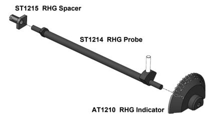
"+1" RHG Spacer position for ride height measuring within 4.0 - 5.2 mm range.
