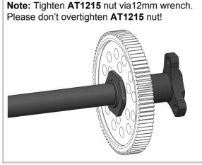
**Note**: The sum of the 64P spur+pinion teeth should be within 112-120 range for short wheel base and within 112-125 range for +1mm longer wheel base.
