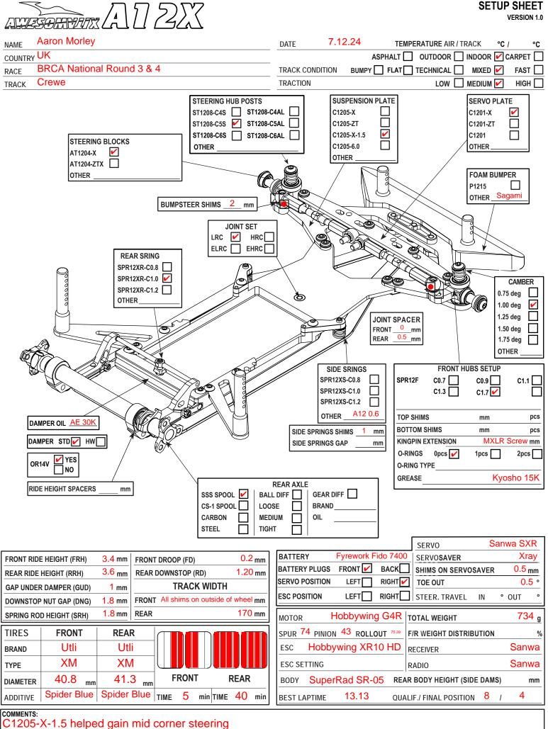
Rear droop was reduced to help settle rear end in direction changes (usually 1.5mm nut gap)
