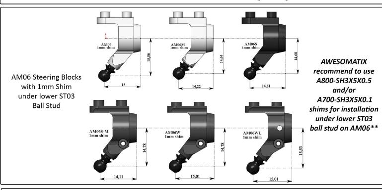
AM06M Steering Block with 1,2mm Shim under lower ST03 Ball Stud
