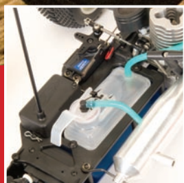
► Large Lever on Floating Fuel Tank
