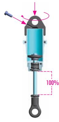
**4** Gently place the shock cap assembly onto the filled shock body. Keep the shock shaft extended 100% from the shock body and tighten the shock cap completely. The rebound will be at approximately 100%.
