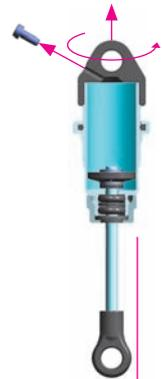
**1** Extend the shock shaft completely and remove the shock cap and remove screw from shock cap.
