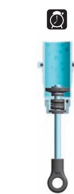
**3** Orient the filled shock vertically for several minutes with the shock shaft fully extended. The remaining air bubbles will release.
