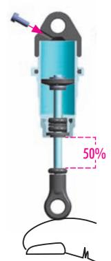
**6** Keep the shock shaft pushed 50% into the shock body and insert the screw into the shock cap. The rebound will be at approximately 50%.
