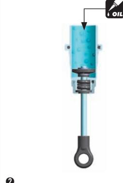
**2** Fill the shock body with shock oil up to the top. Make sure to use same viscosity shock oil as is in the shock.
