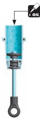
**2** Fill the shock body with shock oil up to the top. Make sure to use same viscosity shock oil as is in the shock.
