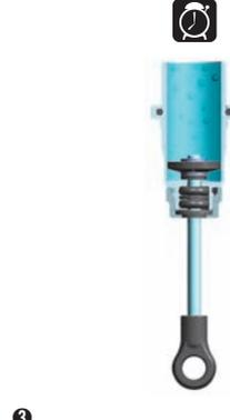
**3** Orient the filled shock vertically for several minutes with the shock shaft fully extended. The remaining air bubbles will release.
