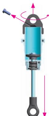
**1** Extend the shock shaft completely and remove the shock cap.
