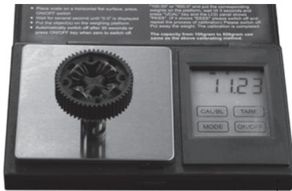
1 Put the diff (without oil) on the scale and check the weight (approximately 11.23g)
