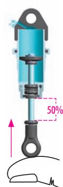
**5** Push the shock shaft 50% into the shock body. Excess oil will bleed through the hole in the shock cap.
