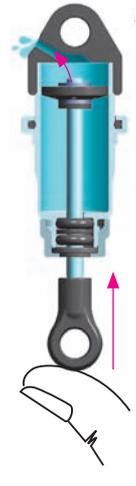
**5** Gently push the shock shaft completely into the shock body. Excess oil will flow through the hole in the shock cap.
