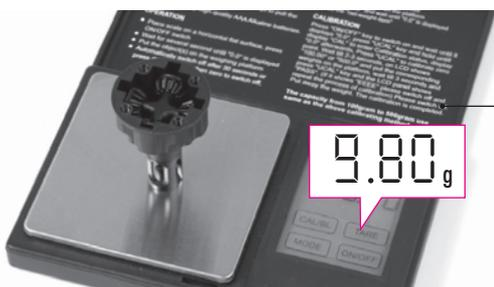
1 Put the diff (without oil) on the scale and check the weight (approximately 9.80g)
