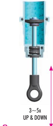
**2** Move the shock shaft up and down a few times to release the air bubbles trapped beneath the piston.
