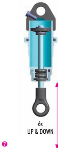
**7** 6x push the shaft up and down.
