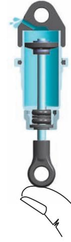
**9** Gently push the shock shaft completely into the shock body. Excess oil will flow through the hole in the shock cap.
