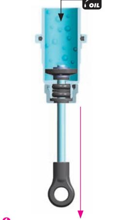
**1** Extend the shock shaft completely. Fill the shock body with the shock oil. For the FRONT shocks (short) use 700cSt oil. For the REAR shocks (long) use 500cSt oil.
