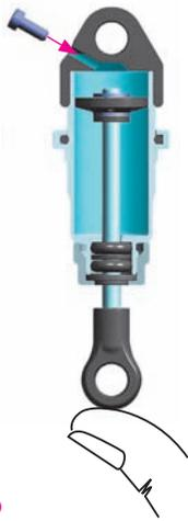
**6** Keep the shock shaft pushed in the shock body and insert the screw into the shock cap. Tighten gently.
