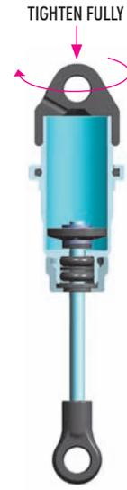
**4** Gently place the shock cap onto the filled shock body and start to tighten the cup. Tighten the cap fully.
