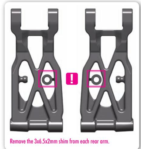
Remove the 3x6.5x2mm shim from each rear arm.
