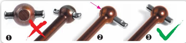
1 Do not use drive shafts when the pins are worn.
