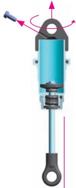
**1** Extend the shock shaft completely and remove the shock cap and remove screw from shock cap.
