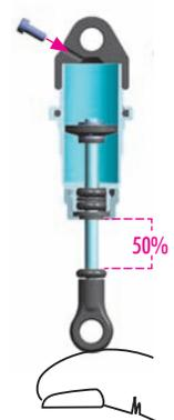
**6** Keep the shock shaft pushed 50% into the shock body and insert the screw into the shock cap. The rebound will be at approximately 50%.
