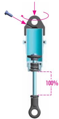
**4** Gently place the shock cap assembly onto the filled shock body. Keep the shock shaft extended 100% from the shock body and tighten the shock cap completely. The rebound will be at approximately 100%.
