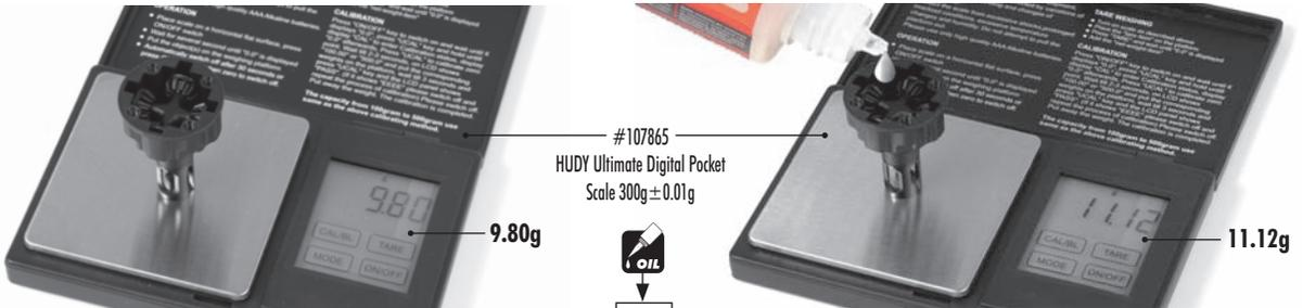
1 Put the diff (without oil) on the scale and check the weight (approximately 9.80g)
