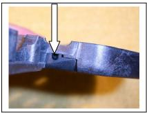
C2 Assemble the motor plate support to the top of the chassis with two 4-40 X 1/4" flat head screws. The screws come up from under the chassis and thread into the support. Notice that the support is off-set to the right and should be installed that way.
