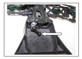
3) Remove the two bolts from under the chassis that hold the servo in, and remove the servo. Leave the servo horn attached to the servo. Remove the four button head screws that hold the servo mount posts (7336) to the servo and save these four screws for re-use. The posts will not be needed.
