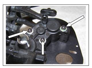
20) From the front of the shock tower (9572), loosen the two flat head screws that hold the wing mounts to the tower.
