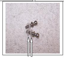
13) From the outside end of the front of the rear control arm (9582), remove the little 2-56 screw that holds in the hinge pin (9622). Don't lose the little screw! Now, from the front of the control arm, use your wrench to push the hinge pin back so you can remove the pin. The hub carrier (9584), with camber link and CVD assembled, will fall off. Save the spacers (4187). Set all these parts – hub carrier assembly, hinge pin, spacer(s) and little screw -- aside for re-use.
