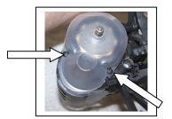
16) Remove the slipper nut (6629), then the spring (9605), slipper plate (9604), slipper pad (9603), spur gear (9651), inside slipper pad (9603), and inside slipper plate (9604). Save all these parts for re-use.
