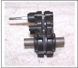
As the case halves come apart, remove and save all of the following parts: Top shaft (9601), spacer (9602), and two 3/8 X 3/16 bearings (6906), Idler gear (9360), two more 3/8 X 3/16 bearings, & idler shaft (9361), ball differential and two ½ X 5/8 outdrive bearings (6903). You will need all the parts from inside the transmission, but the two case halves will not be needed.
