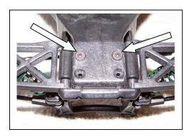
6) From the top of the car, remove the center screw holding the top plate (9566) to the post on the B4 chassis. Save the screw for re-use.
