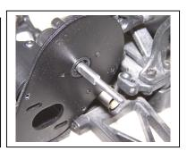
17) From under the car remove the two flat head screws that hold the motor guard (9575). Then, from above, remove the two button head screws that hold the motor guard to the top rear of the transmission (9574). The motor guard and the two button head screws will not be needed. Save the two flat head screws for reuse.
