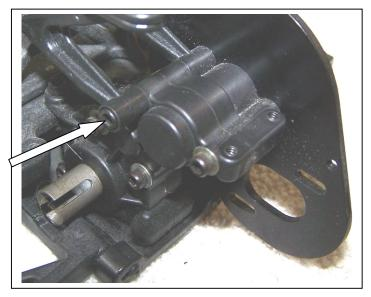
19) Remove the three bolts that go through the transmission and hold the motor plate (9600). These bolts and the plate will not be needed.
