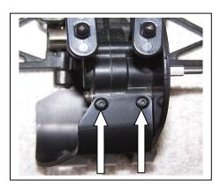
18) Remove the long bolt through the transmission that holds the wing mounts (9587). This bolt will not be needed.
