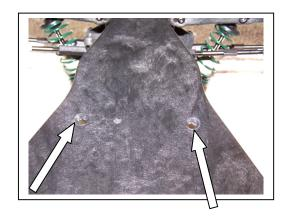
4) Remove the two flat head screws that hold on the front bumper (9562). Take off the bumper. Save it and the two screws for re-use.
