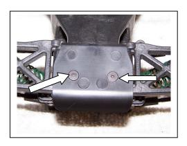
5) Remove the two flat head screws which hold the bulkhead (9563) to the chassis. Save them for re-use.
