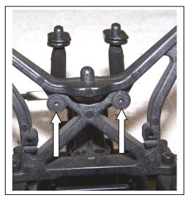
21) From the top, put your wrench down between the wing mounts and remove the two cap head screws that secure the transmission to the shock tower. Now twist the wings mounts a bit and you should be able to remove the transmission from the car. Save the cap head screws for re-use in B2 below.
