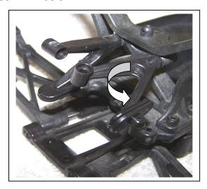
22) Remove the bottom bolt that holds together the two halves of the transmission case and carefully separate the case halves. Save this bolt for re-use.
