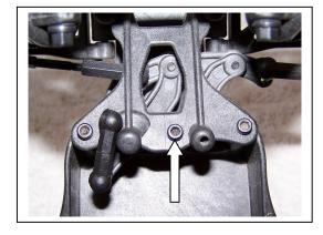
7) Remove the two side top plate screws. Save them for re-use. Carefully remove the front end and steering assembly, and set it aside for re-use. Make sure the steering linkage stays in place.
